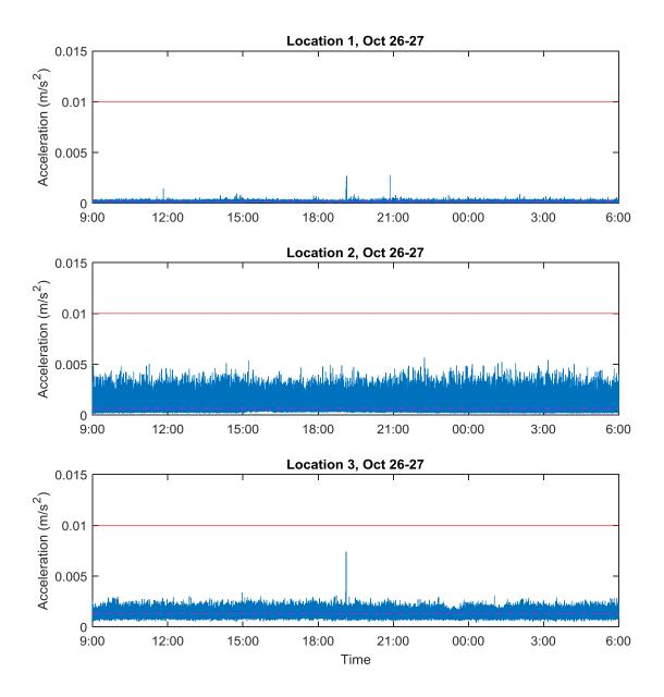
Figure 1: RMS particle accelerations at Location 1, 2 and 3 on October 26-27, 2017. The magenta dash line represents the mean baseline RMS particle acceleration calculated from October 5 to 16 at each location. The red line shows the 0.01 m/s<sup>2</sup> threshold of the RMS particle acceleration.
